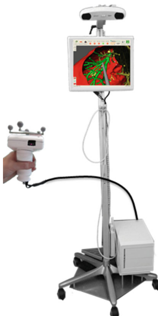
Fig. 3 Stereotactic instrument guidance system with integrated IOD employed within this study
